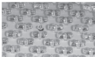
Type I - Long and narrow distribution pattern designed with walkways in mind.
