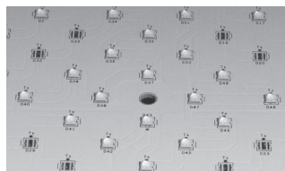
Type V - Symmetrical circle distribution pattern ideal when you need even coverage in all directions.
